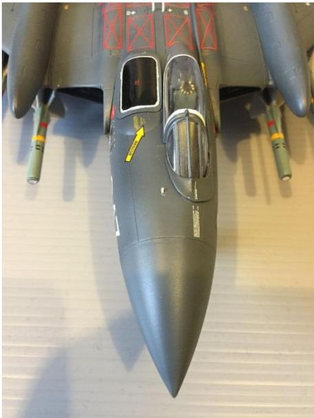
On the FAW.1 version the Observer's Cockpit was covered by a solid metal hatch (with a very small window) flush with the fuselage surface. On the later FAW.2 the hatch was raised slightly to give the observer more headroom, and was a frangible Perspex cover that the observer could eject through. Generally these were painted black on the inside in service, however XP924 currently flying in the UK has this left clear – presumably to make the ride less claustrophobic for any passenger.
