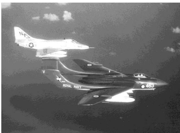
The first squadron of Sea Vixen FAW 1's formed in 1959. The Mark 1 (*left*) was a better looking aircraft (in my extremely humble opinion) which could carry 4 Firestreak missiles, two in-built rocket packs, plus drop tanks. It could carry conventional bombs instead of the Firestreaks.
